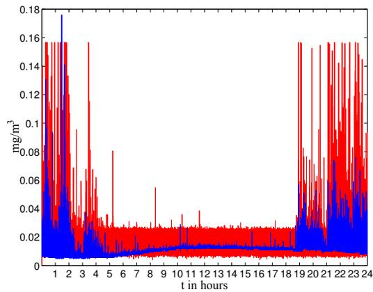
Fig. 3. Data from one of the dust sensors (red curve) and the reference device (blue curve) in  $\frac{mg}{m^3}$ .
