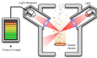
Fig. 1. Many of the sensors use a heating resistor to create an updraft. [11] This limits the possible operation conditions.
