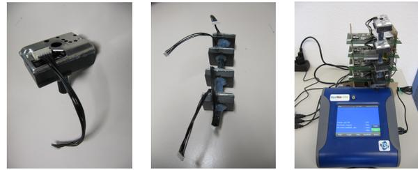
Fig. 2. One of the *Sharp GP2Y1010* optical dust sensors with added hose on the air outlet and four sensors bound together, forming a stack.
