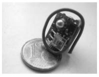
Figure 1: A µPart Sensor Node (1 cm<sup>3</sup> incl. battery)
