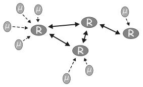
Figure 2: The µPart network topology, consisting of µPart end-nodes and routers
