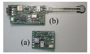
Figure 2. (a) Sensor board with light, temperature, acceleration and microphone sensor, (b) Sensor board with additional microcontroller (backside) and force sensor
