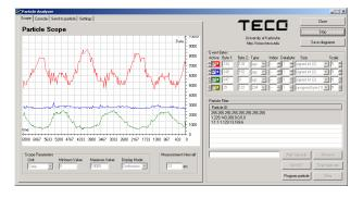
Figure 9. ParticleAnalyzer plotting acceleration data during a rotation of a Particle node
