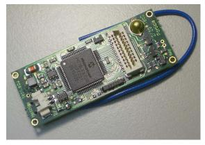
Figure 1. Particle communication board (transceiver, external flash memory, speaker on the backside)
