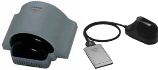
Figure 7. Infrared wireless LAN system
