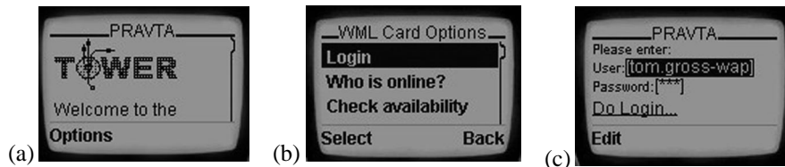
Figure 2. The PRAVTA prototype user interface: (a) front page; (b) action menu list; (c) login dialogue.
