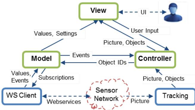
Fig. 2. Overview of the Model-View-Controller system architecture
