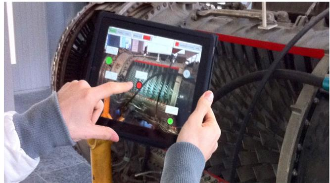
Fig. 3. Interface prototype visualizing data from a sensor equipped turbine
