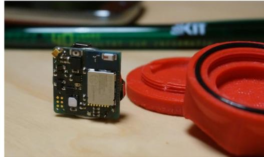
**Figure 1. bPart sensor node (2.1cm x 2.1cm x 0.4cm) next to an industrial grade sensor housing.**
