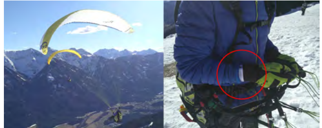
Figure 1. RüttelFlug is a wrist-worn tactile variometer, e.g. for paragliding. It was designed to be unobtrusive and fits well even under thick clothing.
