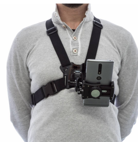
Figure 1. We used a body-worn Tango system to investigate Human Activity Recognition (HAR) using the depth information from the camera.
