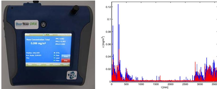
**Fig. 4:** Left: the TSI 8533 DustTrak DRX reference aerosol monitor. Right: data from one of the dust sensors (red curve) and the DustTrak (blue curve) in  $\frac{\text{mg}}{\text{m}^3}$ .
