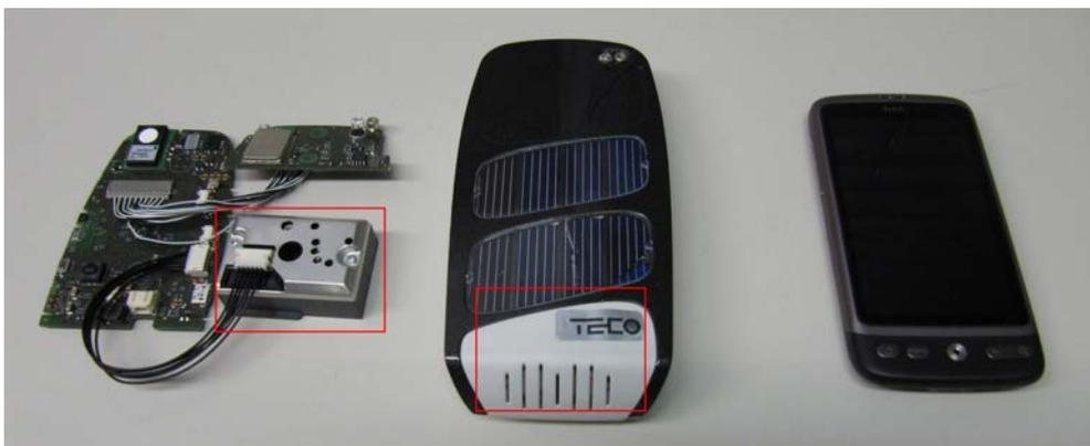
**Fig. 1:** TECO Envboard: PCBs and Sharp dust sensor (left) and in housing (middle).
