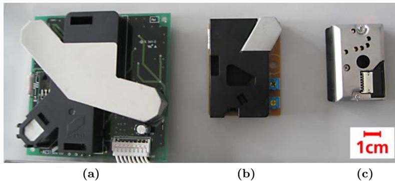
**Fig. 3:** Particulate matter sensors: *AES-1* (a), *DSM501A* (b), and *GP2Y1010* (c).
