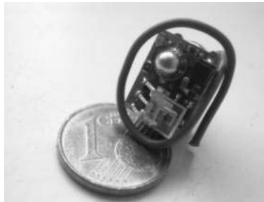
Figure 1: A \mu Part Sensor Node (1 cm 3 incl. battery)
