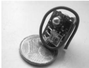
Figure 1: A  $\mu$ Part Sensor Node (1 cm<sup>3</sup> incl. battery)
