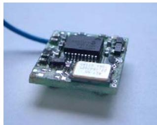
**Fig. 1.** TecO's Particle[7] (1  $\text{cm}^3$  integrating microcontroller, sensors, communication, battery)
