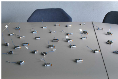
Fig. 11. Prototype implementation of Multi-SDJS on Particle Computers
