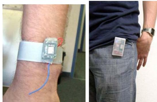
Figure 1: Small Smart-It with sensors attached to body or clothing
