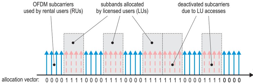
Fig. 1. Schematic example of an OFDM based spectrum pool
