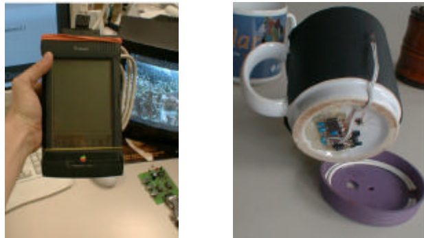
Fig. 6. Two example set-ups of the RAUM system. The left picture shows the PDA with the UbicompBrowser, a PC based network access node and a TV set as controlled device. Right the MediaCup with an IrDA based access point as it is used in the Ambient Telepresence example.
