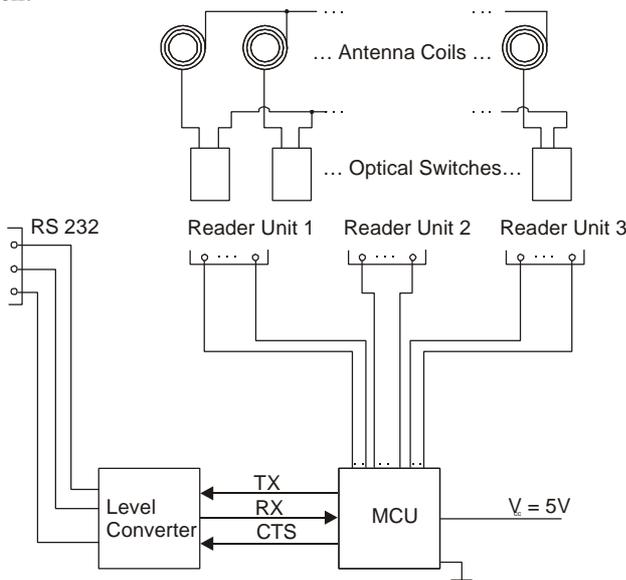
Figure 2. Smart Shelf Schematic.
