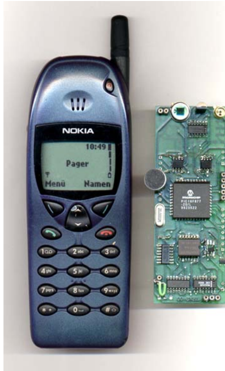
Figure 3. The TEA awareness device was implemented as plug-in for mobile host devices and applied for augmentation of a mobile phone with context relating to so-called profiles.
