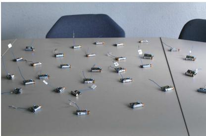
**Fig. 11.** Prototype implementation of Multi-SDJS on Particle Computers
