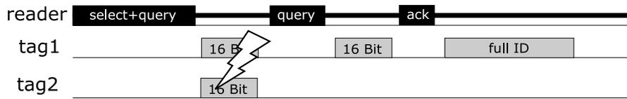
Fig. 5. Using a 16 Bit random number during Identification process
