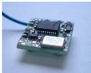
Fig. 1. TecO's Particle[7] (1 \text{cm}^3 integrating microcontroller, sensors, communication, battery)
