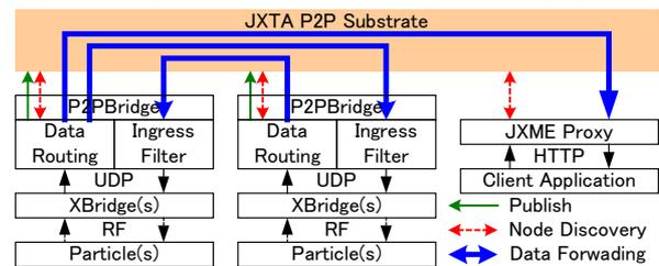
Figure 3. Implemented System Architecture
