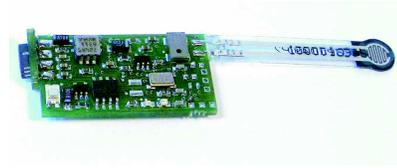
Fig. 7. Particle sensor board
