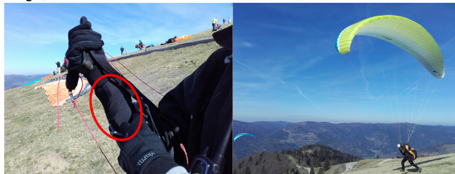
Figure 1: Tactile Variometer worn underneath normal flight gear. The pilots movement is not restricted and the cuff fits under normal clothing. Taken during the evaluation in Fellingring, France.
