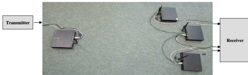
(a) Experimental scenario, relation of the USRP nodes and transmitter and receiver block diagrams
