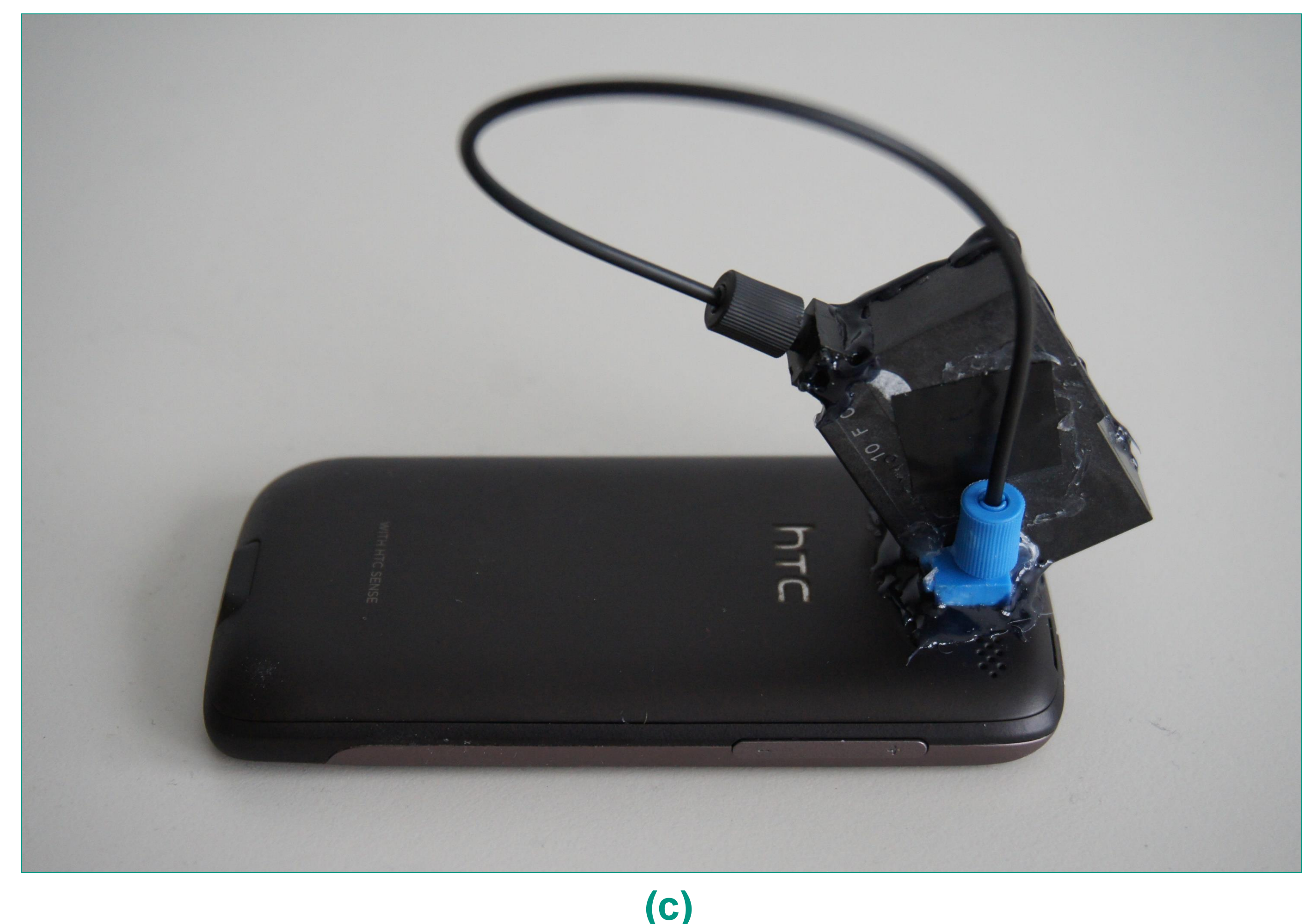
Fig. 1: The Sharp GP2Y1010 dust sensor (a), sketch of our fully passive modification (b) and implementation on a smartphone (c).
