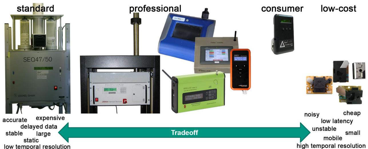
Figure 1. Range of measurement technology (image taken from Budde et al. (2014)<sup>7</sup>).
