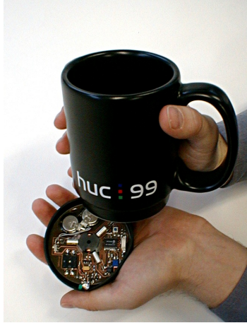
Figure 2: The Mediacup , an early IoT device with sensors to detect movement, temperature and liquid level of the cup [1]. The picture shows the final version from 1999 with wireless recharging.
