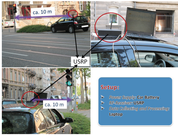
Fig. 1. Experimental setup for the proposed traffic awareness system
