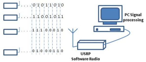
Fig. 3. Principle of collective transmission. Each sensor node reached by an external trigger signal is transmitting its binary sequence at the same time. Based on the different number of '1's in each time slot different maximal amplitudes are generated. On the receiver side, the superimposed binary sequence is captured.
