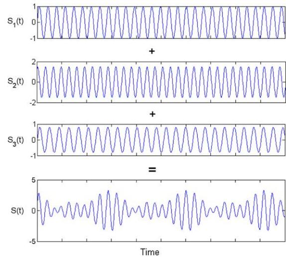
Fig. 4. The superposition principle:  $s(t)$  is a superimposed signal generated by three sine signals  $s_1(t)$ ,  $s_2(t)$  and  $s_3(t)$ . The sine signals are chosen slightly different from each other in frequency, phase and amplitude strength, i.e.  $f_{s_1} = 16$  Hz,  $f_{s_2} = 18$  Hz and  $f_{s_3} = 20$  Hz. Thus, when two or more waves traverse the same space, the amplitude at each point is the sum of the amplitudes of the individual waves.
