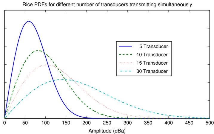
Fig. 9. The four distributions indicate various Rice PDFs obtained by fitting data of 5, 10, 15 and 30 transducers which sent a sinusoidal signal simultaneously.
