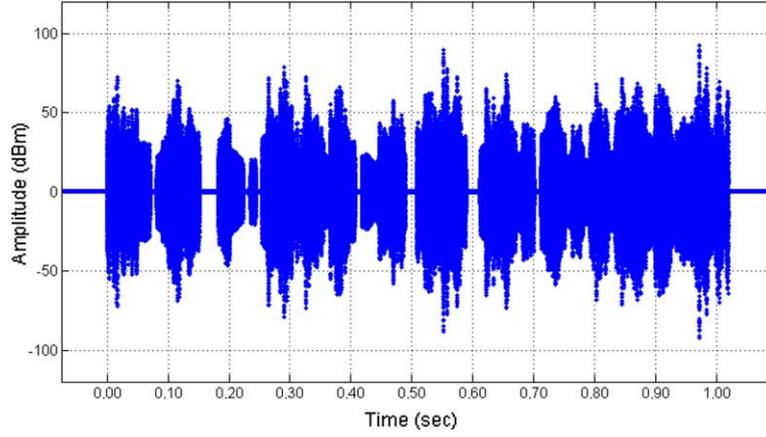
Fig. 5. Raw data of a superimposed signal caused by 21 transducers transmitting different binary sequences simultaneously. The signal length is set to 100 time slots.
