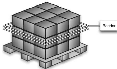
Fig. 1. A typical application scenario for item level tagging in supply chain management: pallets are investigated by a screening device.
