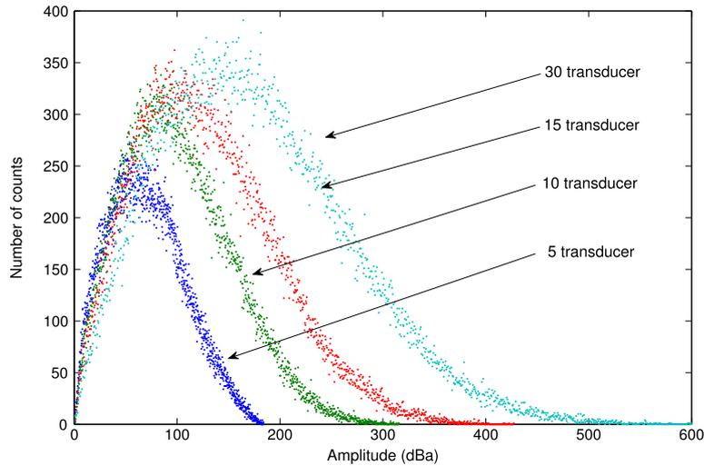
Fig. 8. The four histograms illustrate the distributions of amplitudes which are generated by 5, 10, 15 and 30 transducers sending a sinusoidal signal simultaneously.
