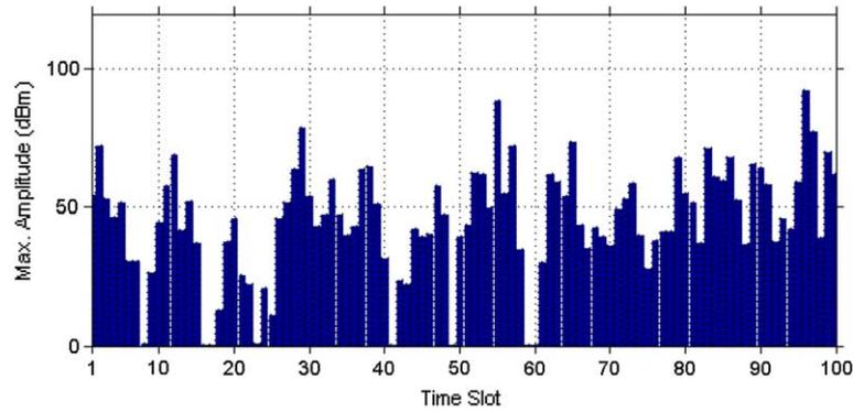
Fig. 6. Quantification of the superimposed signal shown in Fig. 5. In each time slot the maximal amplitude is detected and visualized by a single bar.
