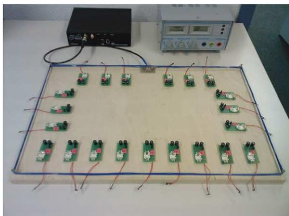
Fig. 7. The research platform consists of 21 transducers and one receiver connected to a PC. During experiments, transducers are controlled by sensor nodes (not shown).
