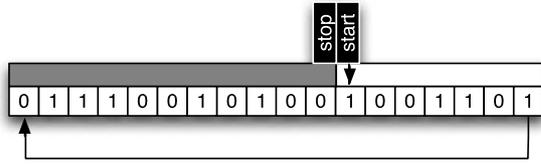
Fig. 2. A model of a simple tag using a destructive, physical temperature sensor (gray and white bar): the start/stop pointer is shifted forward along the fixed random vector  $z_0$  as increasing temperatures permanently alter the material of the sensor (grey). When a read-out signal is received the correspondingly shifted vector would be transmitted.
