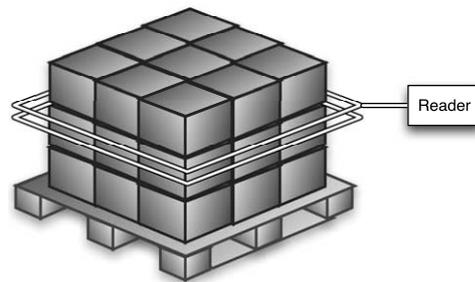
Fig. 1. A typical application scenario for item level tagging in supply chain management: pallets are investigated by a screening device.
