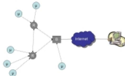
Figure 1. System Architecture with  $\mu$ Part end nodes ( $\mu$ ), router nodes (R) and bridge nodes (B) .
