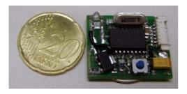
Figure 8: A very low power infrared (IrDA) based location beacon
