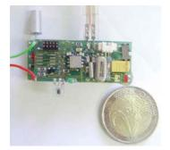
Figure 4. Smart-Its: A general sensing, computing and communication platform to be embedded into everyday artefacts
